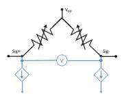
Constant Current Mode: Current level should be chosen for patient safety, signal-tonoise and lifetime requirements. (Blue portions of circuit supplied by customer.) Refer to ISO 60601 for patient risk current safety limits.
