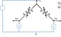
Constant Voltage Mode: Voltage level should be chosen for patient safety, signal-to-noise and lifetime requirements. Refer to ISO 60601 for patient risk current safety limits.
